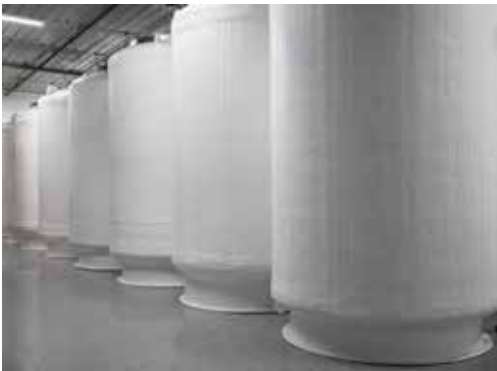
Fig. 1 Cryonics dewars for long-term storage at Cryonics Institute outside Detroit, USA. Photo: Jack Entremont, 2021.
